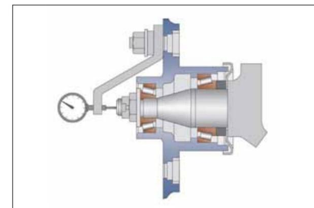
14. Turn the castellated nut back through max. 1/12 turn until it coincides with the next split pin hole and secure with a split pin.
