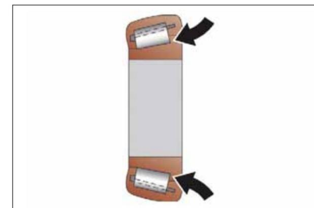
4. Insert the inner ring in the wheel hub.
