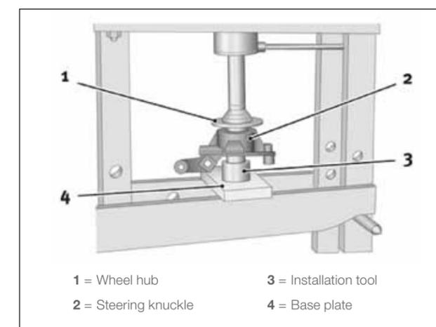
**2.** Tighten the fastening nut of the wheel bearing using the torque recommended by the vehicle manufacturer. The nut torque is not only important for fastening the wheel but also ensures that the wheel bearing runs with the optimum clearance. We urgently recommend using a torque wrench to achieve the right torque.
