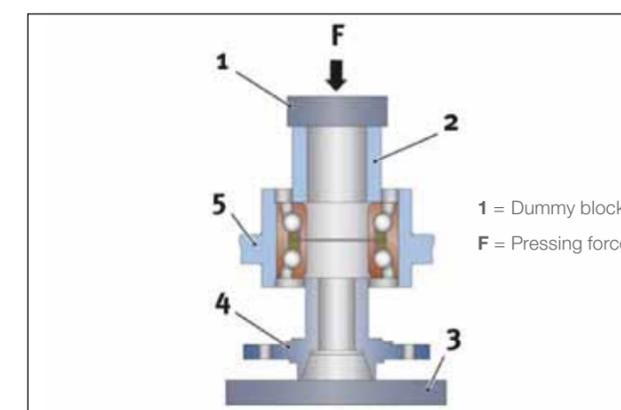
**Note:** in some vehicles, the components are installed in the reverse order. The steering knuckle lies on the base plate and the wheel hub is pressed in from above.
