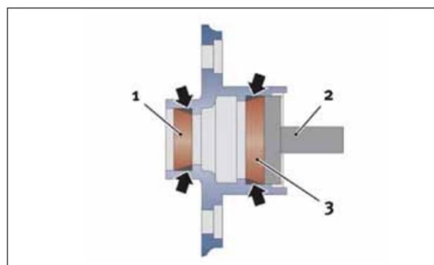
3. Grease the inner ring of the inner bearing well.
