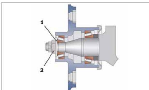
13. Check that the bearing runs correctly with the right tilting clearance.
