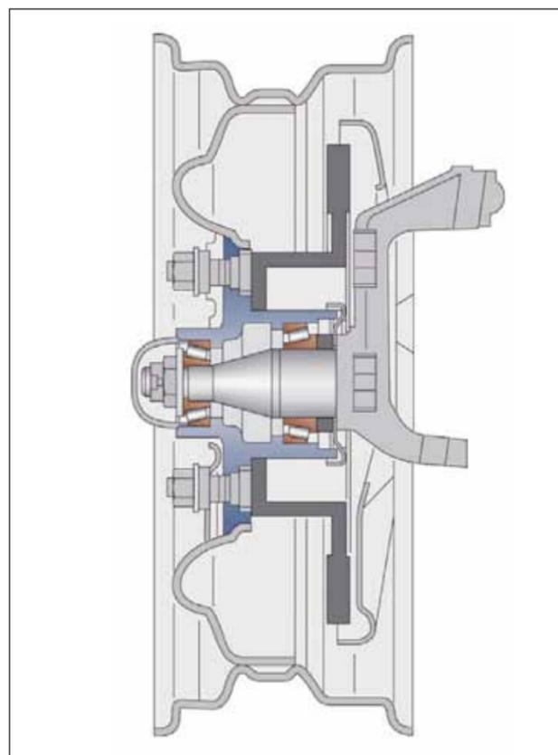
Car bearing with fitted tapered roller bearings (non-driving axle).
